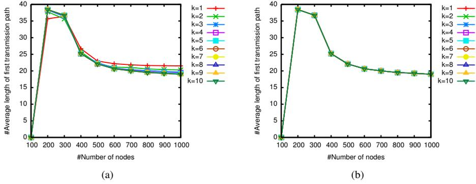
Fig. 4. Average length of the first transmission path explored by TPGF in a CKN based WSN (a) and in an always-on WSN (b).
