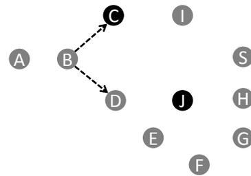
Fig. 1. Latency issue when applying geographic routing in duty-cycled WSNs. Gray nodes are awake nodes and black nodes are asleep nodes. Enroute from A to S, node B should decide waiting for C to wake up or routing from D, E, F, G, H to S. For either decision, the latency may increase significantly.
