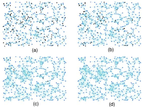
Fig. 3. One example of a CKN based WSN with different  $k$ . There are total 500 nodes and the  $k$  in CKN is 1, 2, 4, 8 in (a) (b) (c) (d), respectively. The red node is the source node and the green node is the sink node. The black nodes are asleep nodes and the blue nodes are awake nodes. The line between two nodes means they are neighbors. When the  $k$  in CKN increases, the number of asleep nodes decreases.
