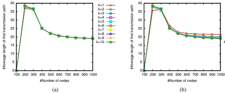
Fig. 5. Average length of the first transmission path explored by TPGF in GSS based WSNs (a) and CKN based WSNs (b).
