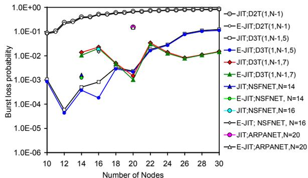
Fig. 8. Burst loss probability, as a function of the number of nodes ( $N$ ), in the last hop of rings, degree-three chordal rings, FCCN-NET, NSFNET, and ARPANET, for JIT and E-JIT protocols;  $\lambda/\mu=32$ ;  $F=64$ ;  $T_{Setup}(JIT)=T_{Setup}(E-JIT)=12.5\mu s$ .
