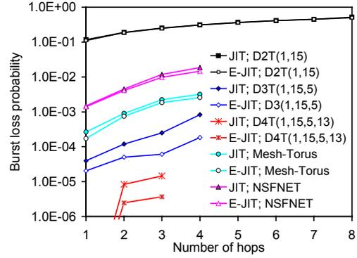
Fig. 6. Burst loss probability, as a function of number of number of hops, for ring (D2T(1,15)), chordal ring (D3T(1,15,5) and D4T(1,15,5,13)), NSFNET, and Mesh-Torus networks using JIT and E-JIT protocols;  $\lambda/\mu=32$ ;  $F=64$ ;  $N=16$ ;  $T_{Setup}(JIT)=T_{Setup}(E-JIT)=12.5\mu s$ .
