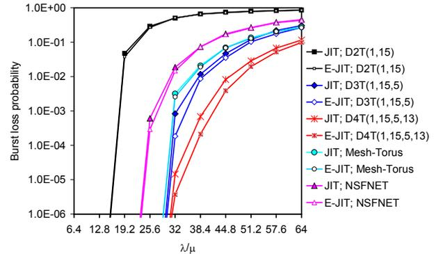
Fig. 7. Burst loss probability, as a function of  $\lambda/\mu$ , in the last hop ring (D2T(1,15)), chordal ring (D3T(1,15,5) and D4T(1,15,5,13)), NSFNET, and Mesh-Torus networks for JIT and E-JIT protocols;  $F=64$ ;  $N=16$ ;  $T_{Setup}(JIT)=T_{Setup}(E-JIT)=12.5\mu s$ .
