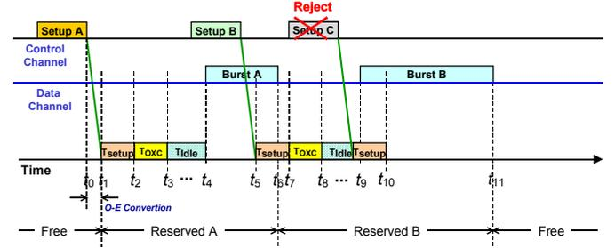
Fig. 3. Operation of E-JIT resource reservation protocol (rejecting a burst).
