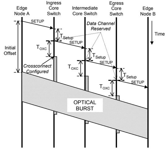
Fig. 1. Schematic representation of E-JIT signaling messages for a successful burst transmission.
