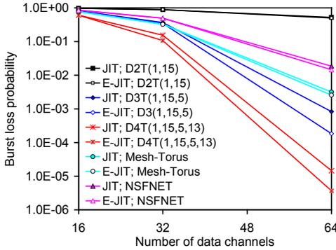
Fig. 5. Burst loss probability, as a function of number of number of data channels per link ( $F$ ), in the last hop of ring (D2T(1,15)), chordal ring (D3T(1,15,5) and D4T(1,15,5,13)), NSFNET, and Mesh-Torus networks for JIT and E-JIT protocols;  $\lambda/\mu=32$ ;  $N=16$ ;  $T_{Setup}(JIT)=T_{Setup}(E-JIT)=12.5\mu s$ .
