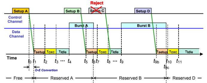
Fig. 4. Operation of E-JIT resource reservation protocol (accepting a new burst).
