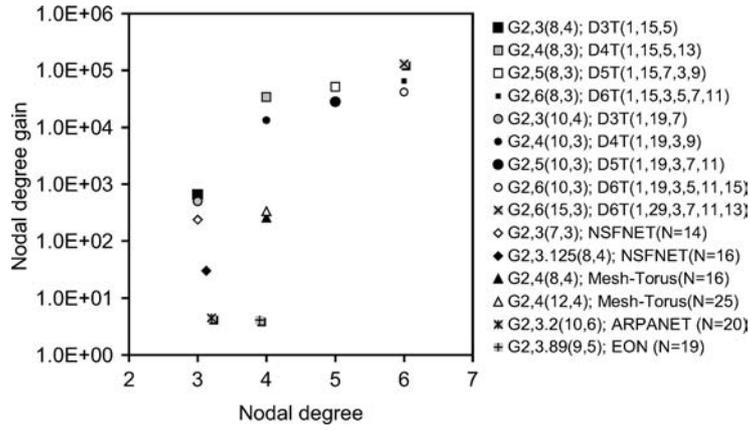
Figure 11. Nodal degree gain in the last hop of each topology, as a function of the nodal degree for Horizon resource reservation protocol;  $\lambda/\mu = 32$ ;  $F = 64$ .
