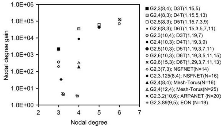
Figure 8. Nodal degree gain in the last hop of each topology, as a function of the nodal degree for JumpStart resource reservation protocol;  $\lambda/\mu = 32$ ;  $F = 64$ .
