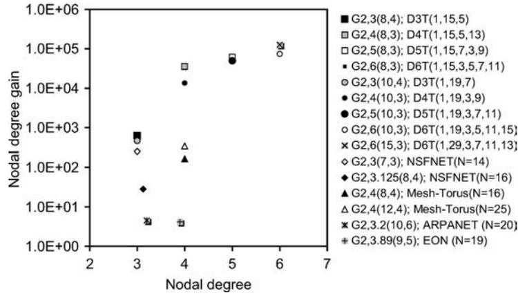
Figure 7. Nodal degree gain in the last hop of each topology, as a function of the nodal degree for JIT resource reservation protocol;  $\lambda/\mu = 32$ ;  $F = 64$ .
