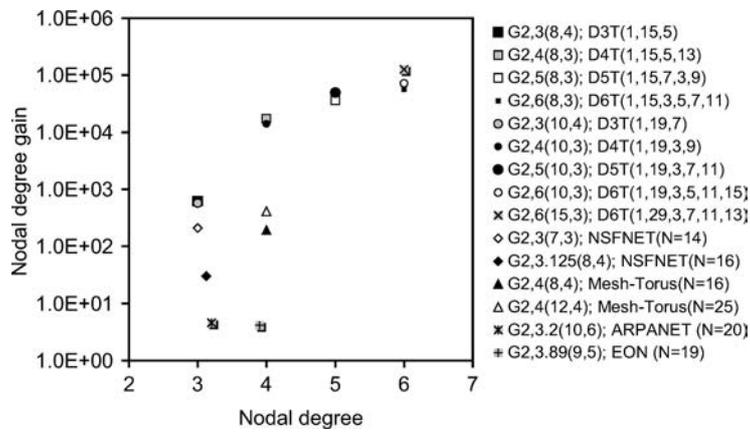
Figure 10. Nodal degree gain in the last hop of each topology, as a function of the nodal degree for JET resource reservation protocol;  $\lambda/\mu = 32$ ;  $F = 64$ .
