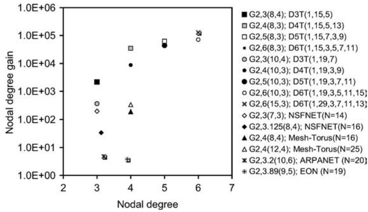
Figure 9. Nodal degree gain in the last hop of each topology, as a function of the nodal degree for JIT<sup>+</sup> resource reservation protocol;  $\lambda/\mu = 32$ ;  $F = 64$ .
