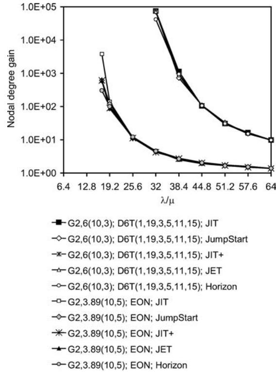
Figure 6. Nodal degree gain due to the increase of the nodal degree from 2 (D2T(1,19)) to: 3.89 (EON), and 6 (D6T(1,19,3,5,11,15)), as a function of  $\lambda/\mu$ , in the last hop of each topology, for JIT, JumpStart, JIT<sup>+</sup>, JET, and Horizon protocols;  $N = 20$ ,  $F = 64$ .
