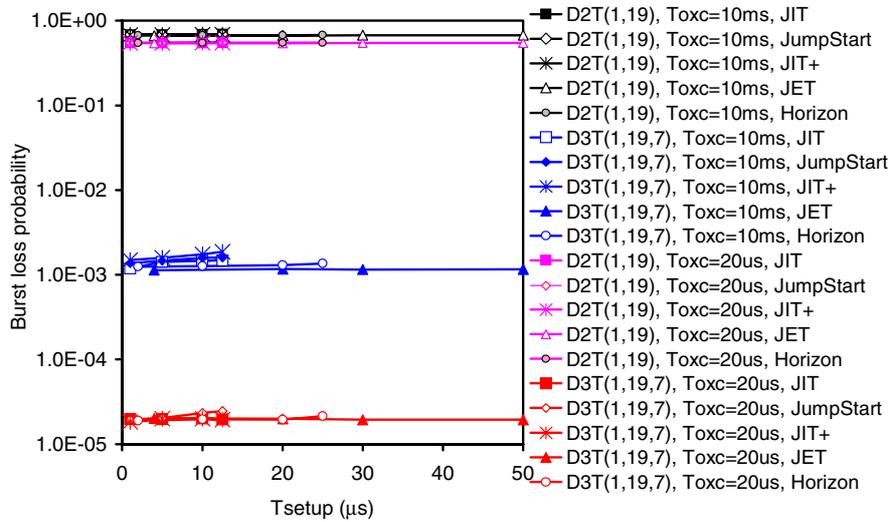
**Fig. 2.** Burst loss probability as function of Setup processing time in the last hop of D2T(1,19) and D3T(1,19,7) for JIT, JumpStart, JIT<sup>+</sup>, JET, and Horizon;  $F=64$ ;  $\lambda/\mu=32$
