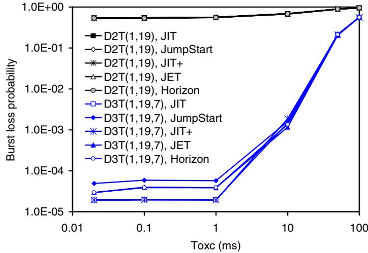
**Fig. 1.** Burst loss probability as function of OXC configuration time in the last hop of D2T(1,19) and D3T(1,19,7) for JIT, JumpStart, JIT<sup>+</sup>, JET, and Horizon;  $F=64$ ;  $\lambda/\mu=32$ ;  $T_{Setup}(JIT)=T_{Setup}(JumpStart)=T_{Setup}(JIT^+)=12.5\mu s$ ;  $T_{Setup}(JET)=50\mu s$ ;  $T_{Setup}(Horizon)=25\mu s$ .
