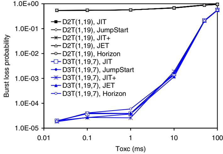
**Fig. 3.** Burst loss probability as function of OXC configuration time in the last hop of D2T(1,19) and D3T(1,19,7) for JIT, JumpStart, JIT<sup>+</sup>, JET, and Horizon; F=64;  $\lambda/\mu=32$ ; with varied  $T_{Setup}$  according to (1), (2), and (3) for each resource reservation protocol
