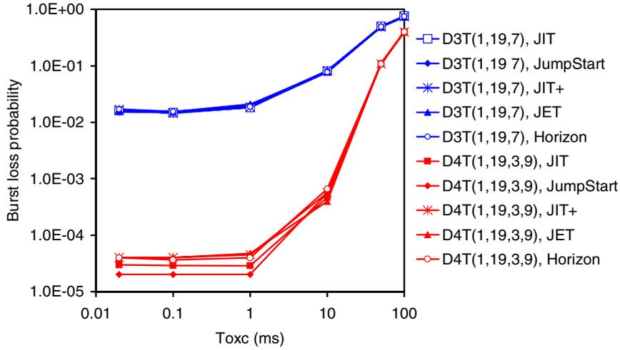
**Fig. 4.** Burst loss probability as function of OXC configuration time in the last hop of D3T(1,19,7) and D4T(1,19,3,9) for JIT, JumpStart, JIT<sup>+</sup>, JET, and Horizon;  $F=64$ ;  $\lambda/\mu=44.8$ ; with varied  $T_{Setup}$  according to (1), (2), and (3) for each resource reservation protocol
