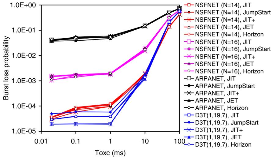
**Fig. 5.** Burst loss probability as function of OXC configuration time in the last hop of NSFNET ( $N=14$ ), NSFNET ( $N=16$ ), ARPANET, and D3T(1,19,7) for JIT, JumpStart, JIT<sup>+</sup>, JET, and Horizon;  $F=64$ ;  $\lambda/\mu=32$ ;  $T_{Setup}(JIT) = T_{Setup}(JumpStart) = T_{Setup}(JIT^+) = 12.5\mu s$ ;  $T_{Setup}(JET)=50\mu s$ ;  $T_{Setup}(Horizon)=25\mu s$
